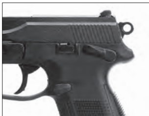
Hammer decocked for double-action firing
