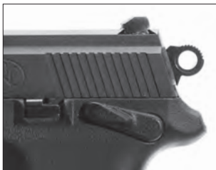
The ambidextrous “safety”/decocking lever shown in the on safe position.
